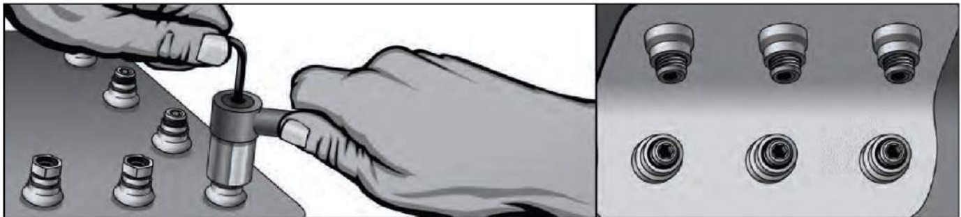
Installing the Hi-Lok® fastener with the "Roller Clutch" wrench.
